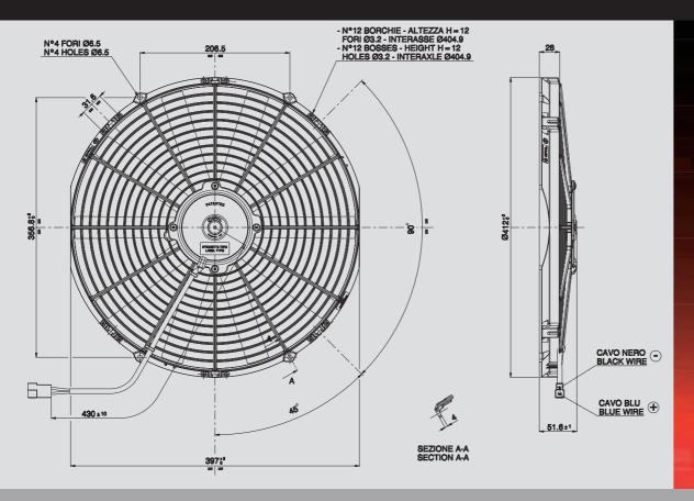
Suggested mounting torque: 3(+1/-0) Nm with screw M5 Weight 1,3 Kg. approx.
